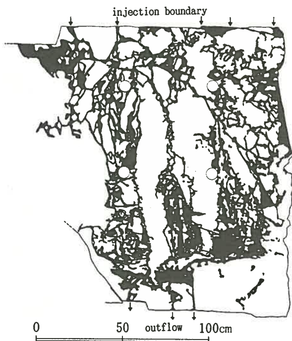
Fig.1 The Channel through the In-situ Single Discontinuity (KIKUCHI et al.)
