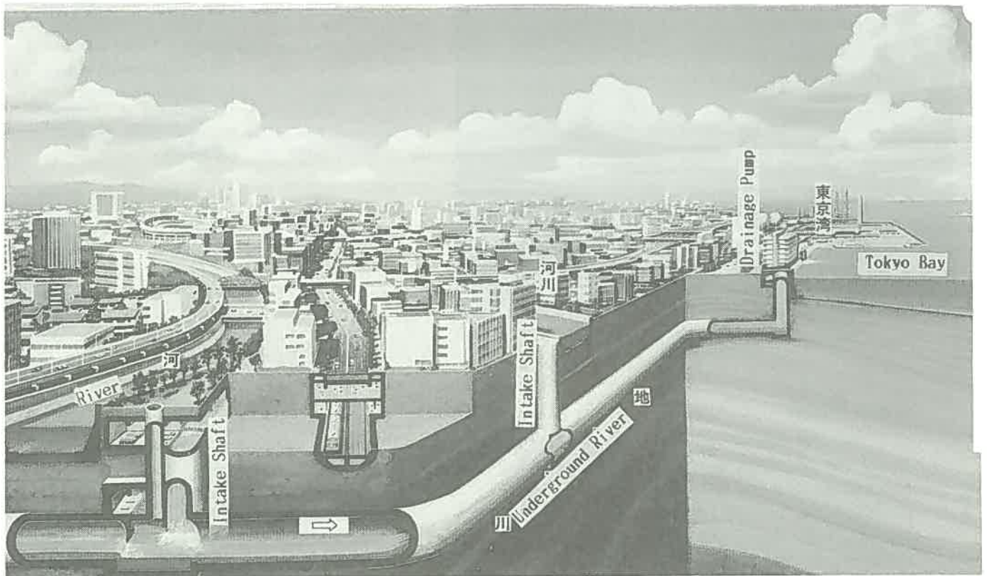
Fig.3 Image picture of underground river system in Tokyo
