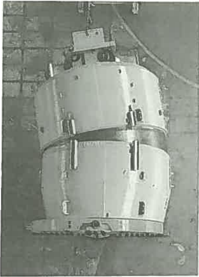
Fig.10 Articulate Shield for Curve Setting
